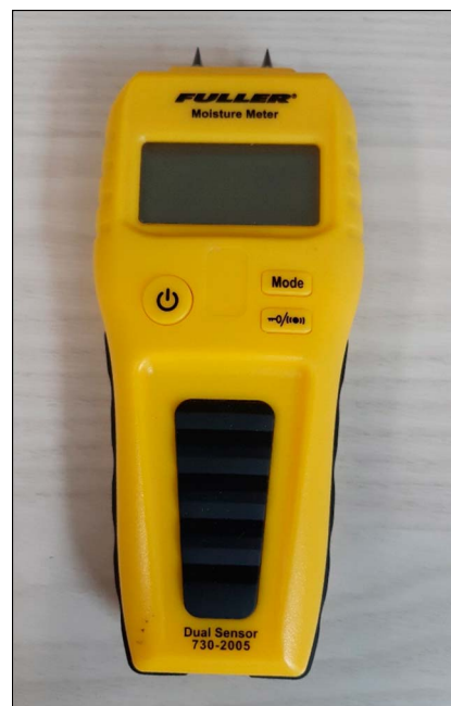
Photograph showing Fuller moisture meter, model 730 to 2005 used in experiment.
